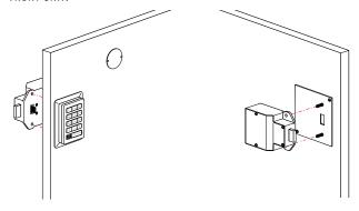
NOTE: DO NOT TOUCH THE REAR UNIT CONNECTOR PINS (MALE CONNECTOR) AGAINST ANY METAL OR OTHER CONDUCTIVE SURFACES. THIS MAY SHORT THE PINS AND CAUSE DAMAGE TO THE LOCK.
