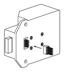
NOTE: DO NOT TOUCH THE REAR UNIT CONNECTOR PINS (MALE CONNECTOR) AGAINST ANY METAL OR OTHER CONDUCTIVE SURFACES. THIS MAY SHORT THE BATTERIES AND CAUSE DAMAGE TO THE LOCK.
